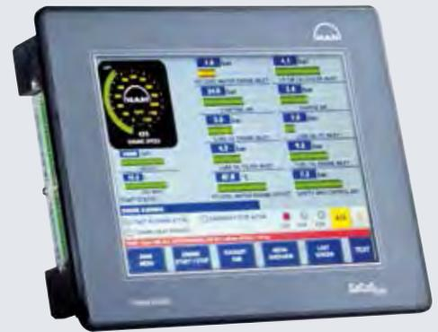
It also connects the control unit to the GenSet, the ship's alarm system and the optional crankcase monitoring system.
